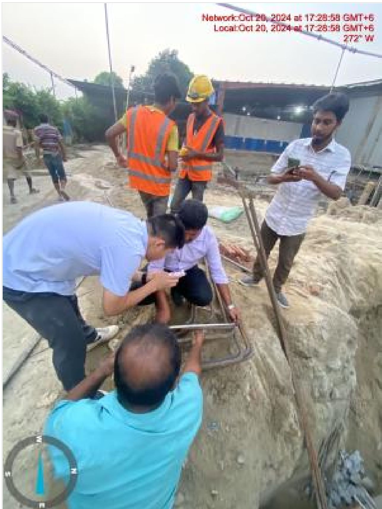
PIT (Pile Integrity) testing on 20-10-24
